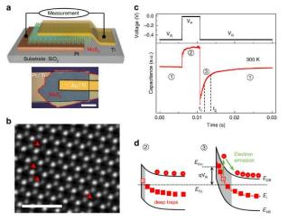
(a) Schematic and optical image MoS2 device for DLTS. (b) STEM image of Sulfur-vacancies in a monolayer MoS2 flake. (c) Capacitance transient (bottom) in response to a pulsed change in bias voltage (top). (d) Band bending of the Schottky junction (MoS2/Pt), illustrating the electron trapping and emission process. Figure from [2].
